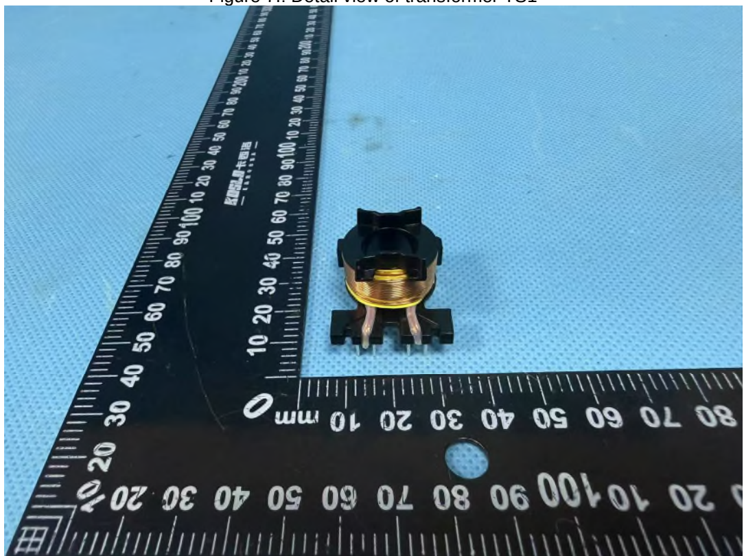
Figure 8.: Detail view of transformer TS1
