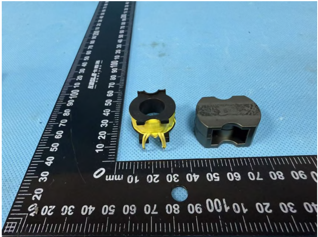
Figure 7.: Detail view of transformer TS1
