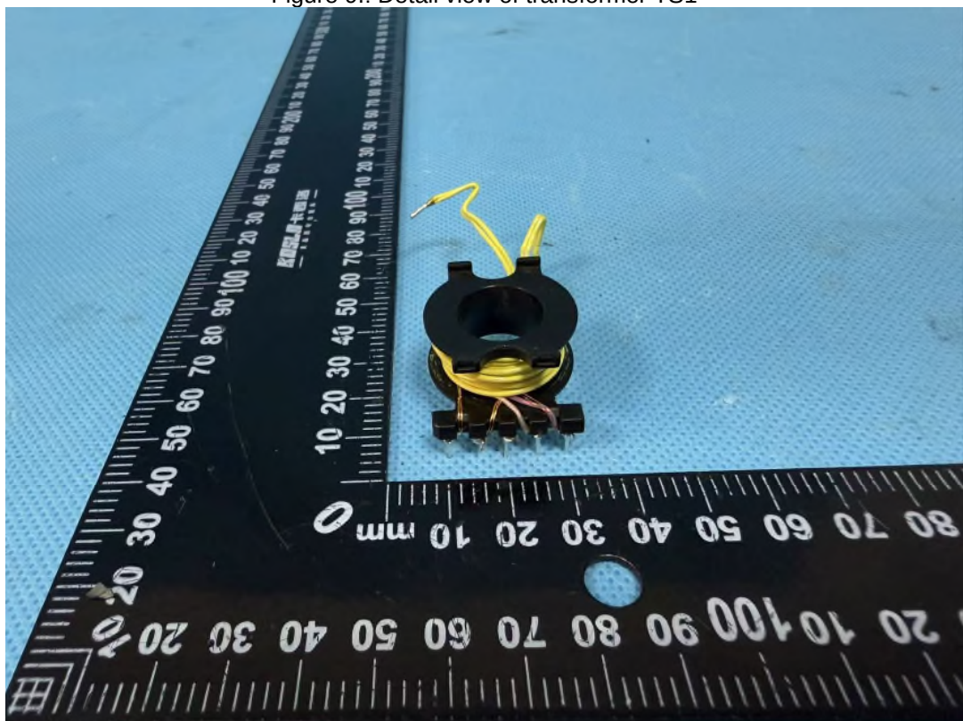
Figure 10.: Detail view of transformer TS1
