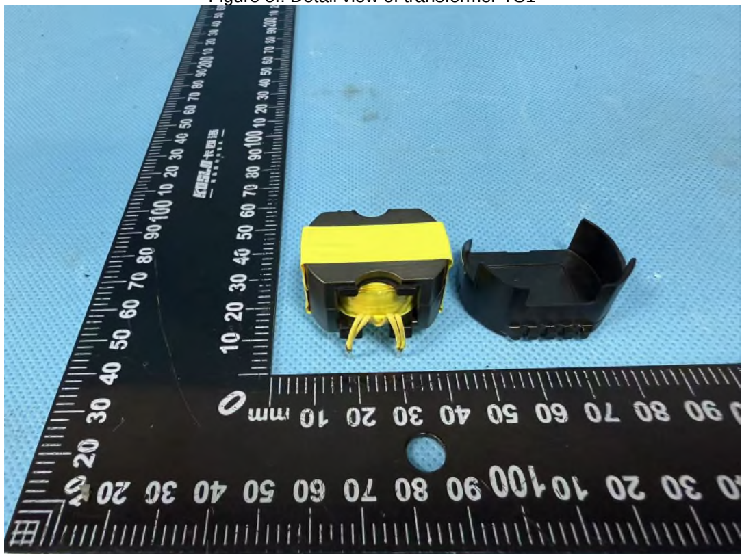
Figure 6.: Detail view of transformer TS1
