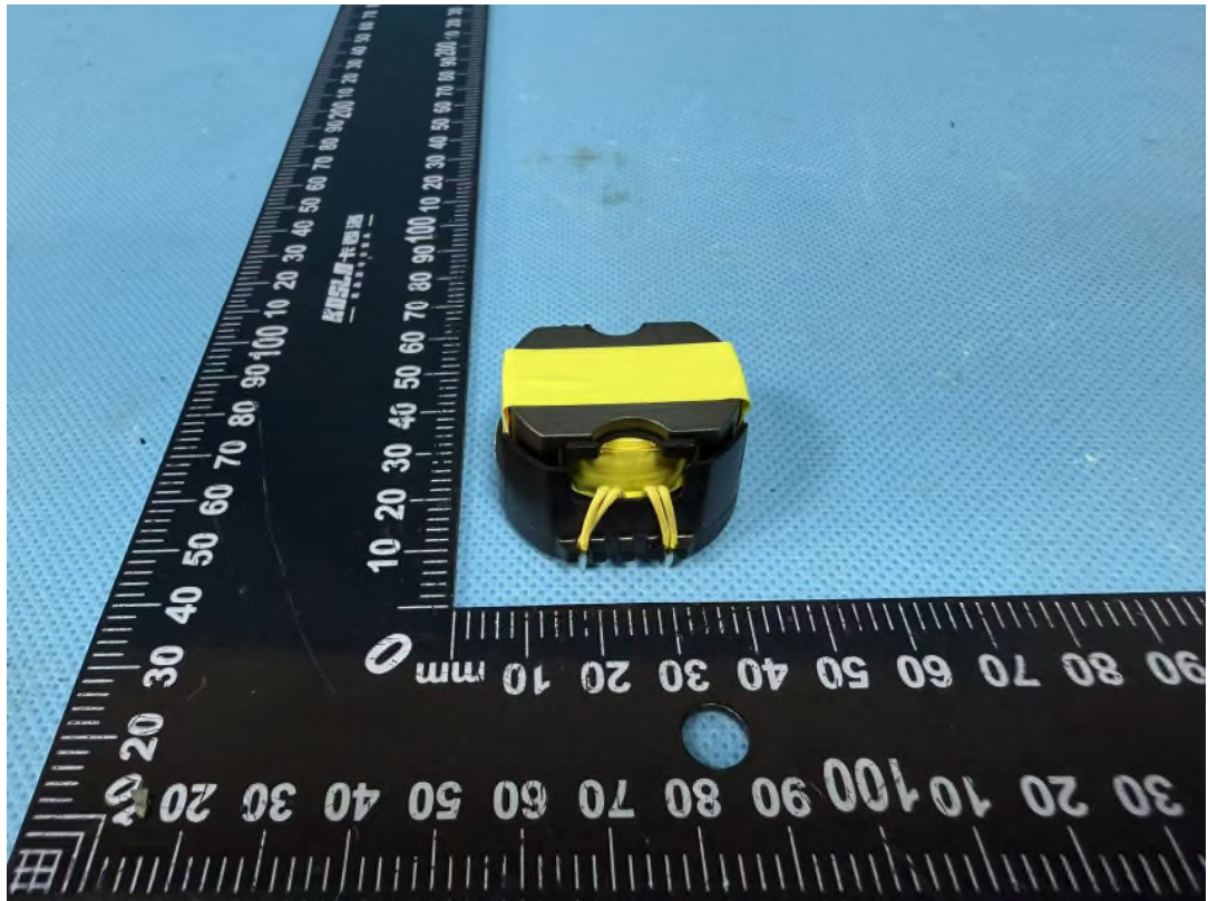
Figure 5.: Detail view of transformer TS1
