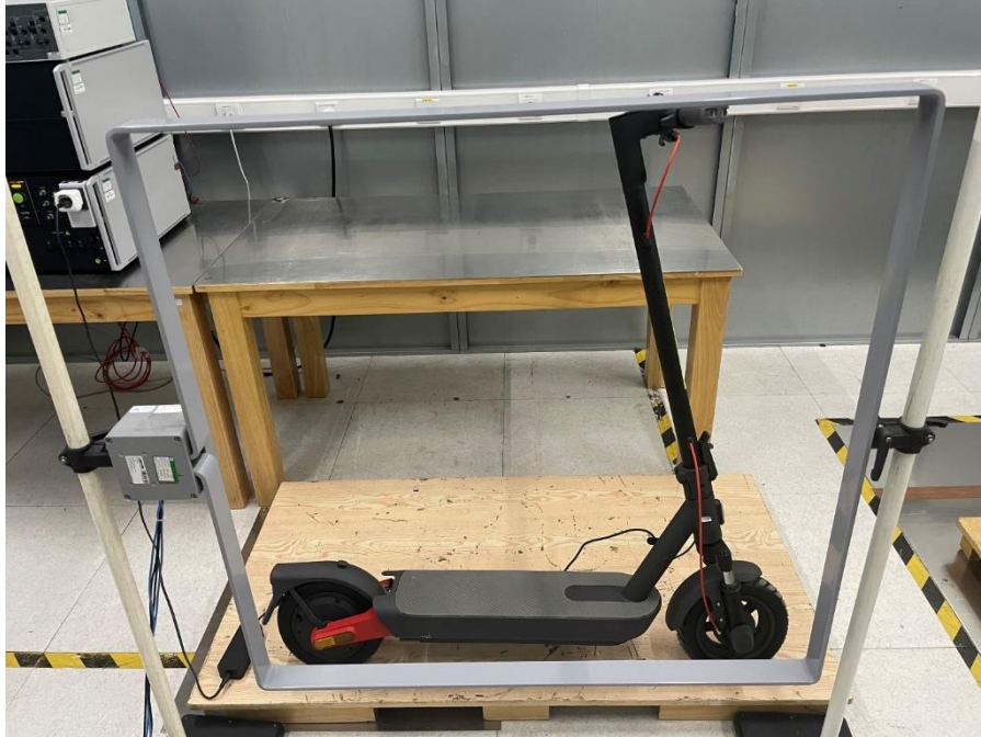
Photograph 5: Set-up for Power-Frequency Magnetic Field
