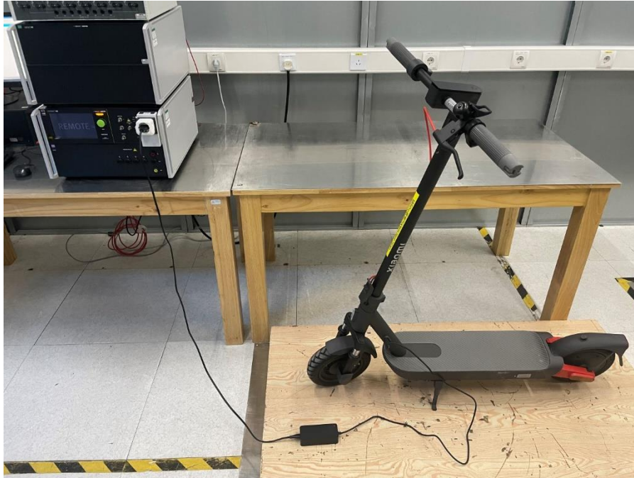
Photograph 10: Set-up for EFT & Surge & Voltage Dips and Interruptions
