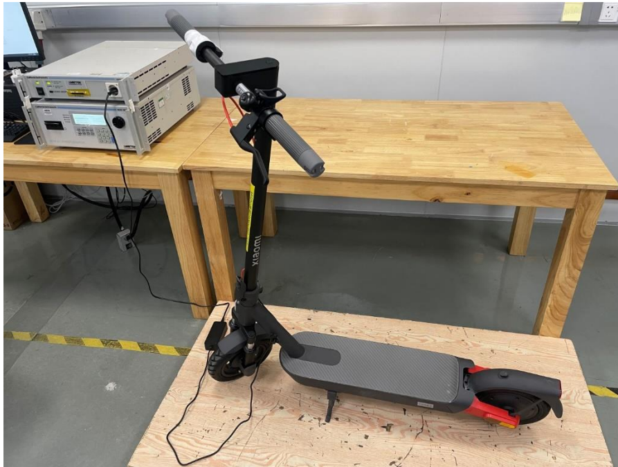
Photograph 1: Set-up for Voltage Fluctuations and Current Harmonics
