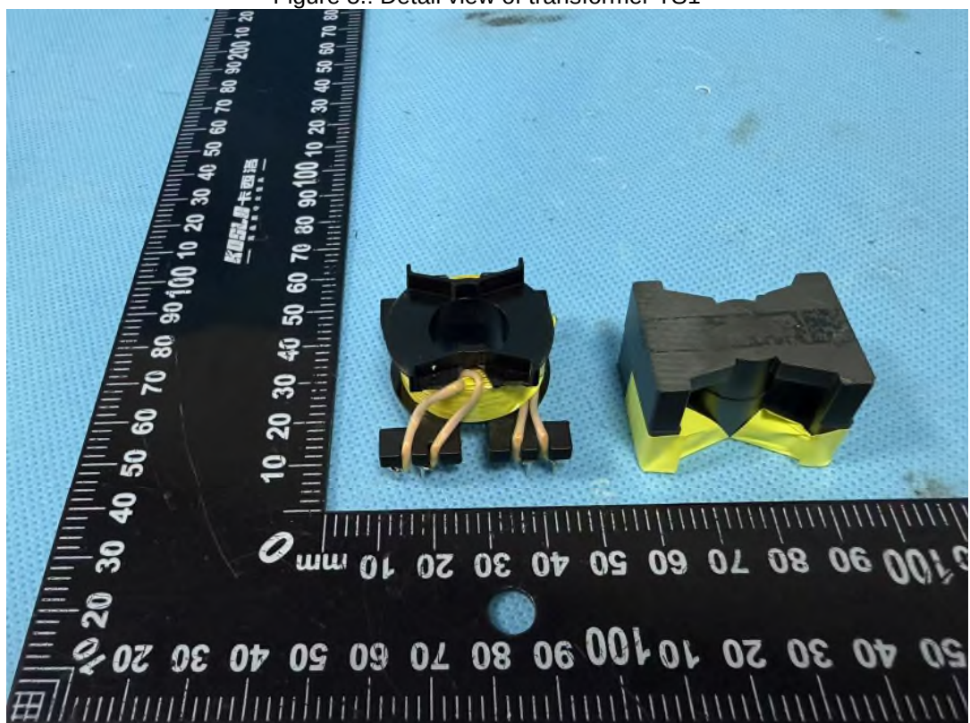
Figure 6.: Detail view of transformer TS1
