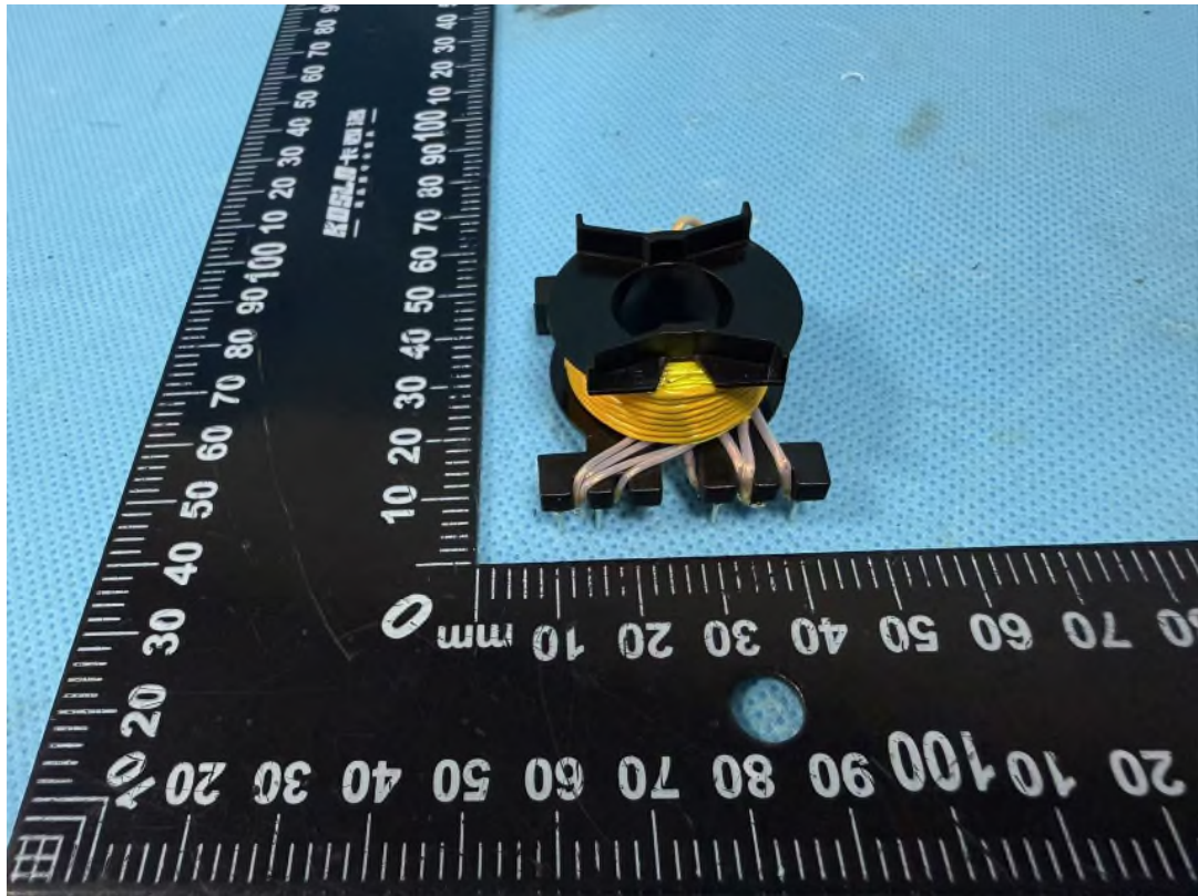
Figure 7.: Detail view of transformer TS1
